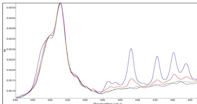
Figure 3. FT-Raman spectra for placebo (purple curve) and EVA/E2 extrudates containing 0.3% (green curve), 2.5% E2 (red curve), or 10% E2 (blue curve) between 680 and 470  $\text{cm}^{-1}$ .
