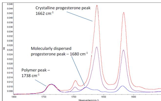
Figure 2. FT-Raman spectra of EVA/P extrudates containing 5% P (blue curve), 15% P (purple curve) and 27% P (red curve) between 1800 and 1500  $\text{cm}^{-1}$ .
